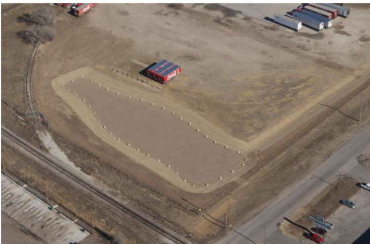
Large, natural stones along the border define the no-mow rain garden bed. Erosion control blanket protects soil on the banks.
